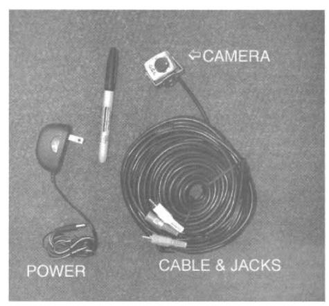
The camera equipment used in the observation box, to bring live images to a television screen. The pen is in the picture for size comparison.
