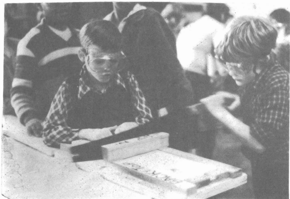
A special jig is used to cut the top and back of the box.
