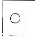
Predator Guard (5 3/8" x 5 3/8"); Drill 1 1/2" or 1 9/16" entrance hole after mounting predator guard on door piece.
