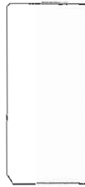
Back (5 3/8" x 11 1/8); Trim 1/4" off one entire end piece to provide for cross venting.
